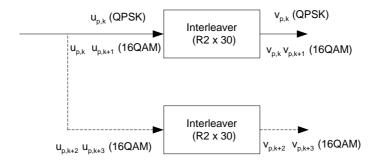
Figure 8a: Interleaver structure for Secondary CCPCH
